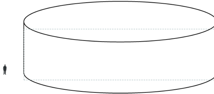
Figure 19. Half-symmetry tank domain used for the parametric study. The tank is 9.8 m (32 ft) high with a diameter of 38 m (126 ft) and an initial water height of 4.9 m (16 ft).
