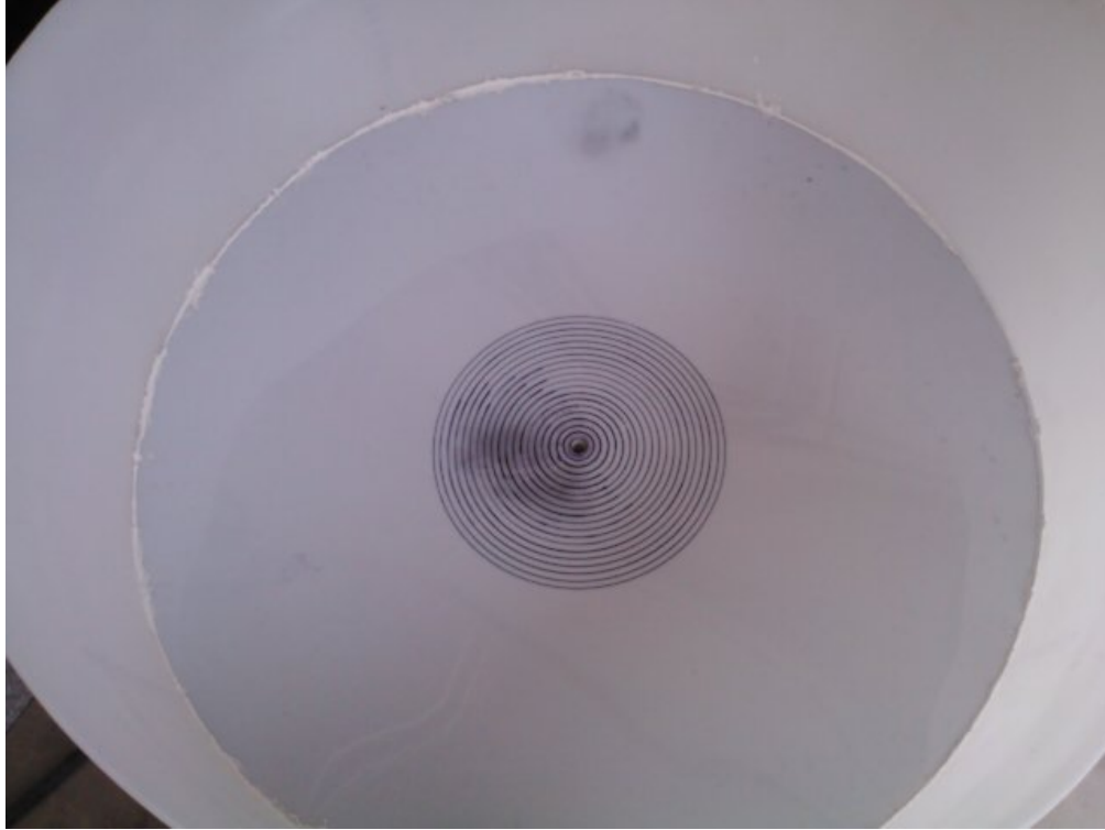
Figure 36. Top view of the bottom of the experimental tank. The inlet/drain line can be seen in the middle, surrounded by concentric circles. The circles were drawn 1 cm apart from each other for spatial reference during the particle resuspension tests.
