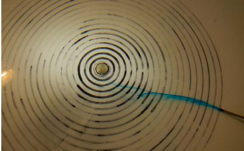
Figure 43. Tracer testing during draining. Note: Each ring is one centimeter apart.
