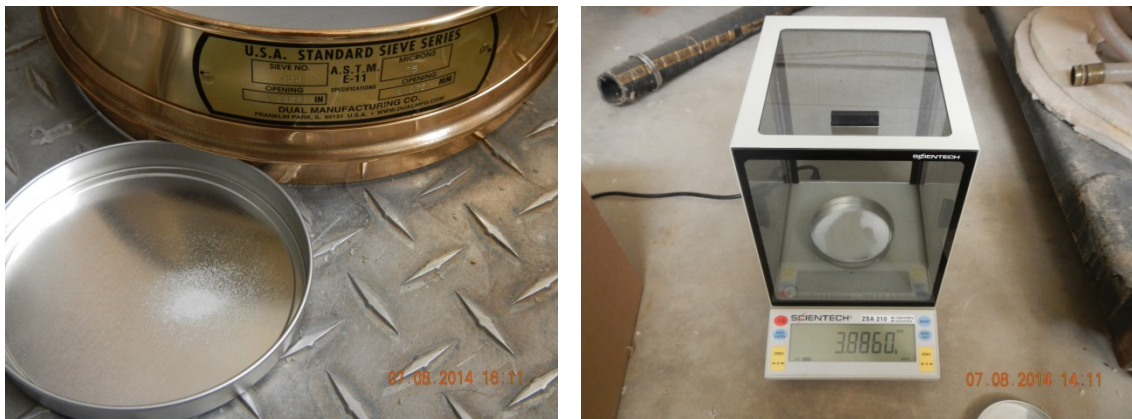
Figure 41. Dried particles from sieve were poured into containers (left) and weighed using a Scientech ZSA 210 scale (right).
