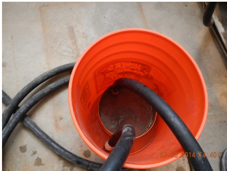
Figure 39. Drained particles collected in sieve.
