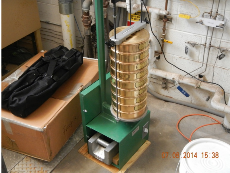
Figure 40. Dried particles were sorted by size using a sieve shaker (Dual H-4325).
