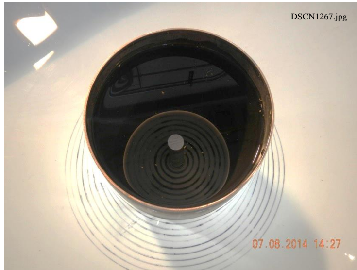
Figure 37. Cylinder used to restrict particles during particle emplacement.
